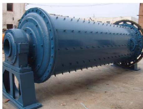
Replacement 3.5t/hr ball mill awaiting inspection in Zhengzhou, China
